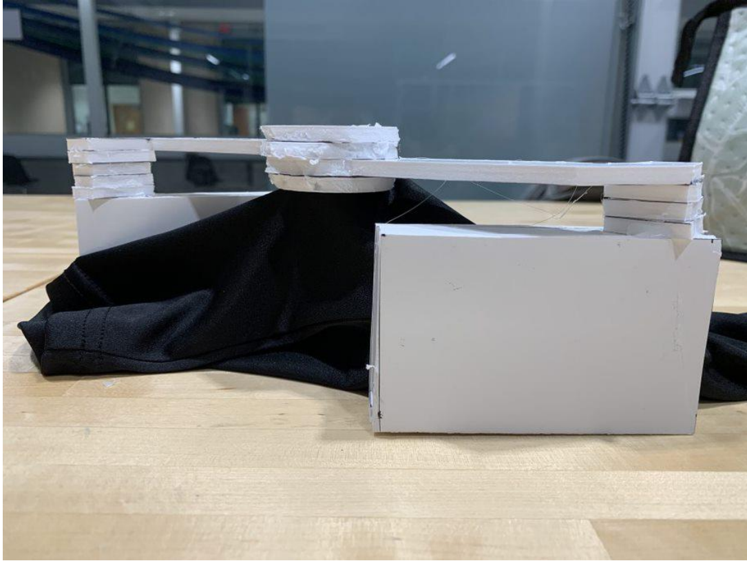
Sideview of prototype, note the differentiation of arm height and such 3 vs 4 risers being used. Also note the attachment of arms to boxes relative to the center of the box.
