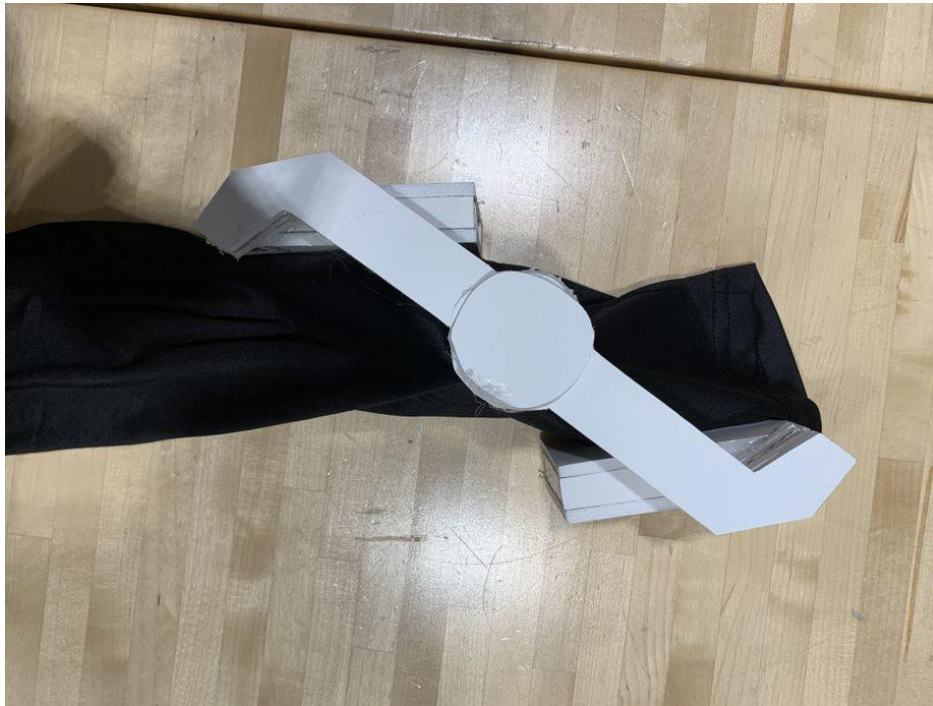
Sideview of prototype, note the differentiation of arm height and such 3 vs 4 risers being used. Also note the attachment of arms to boxes relative to the center of the box.
