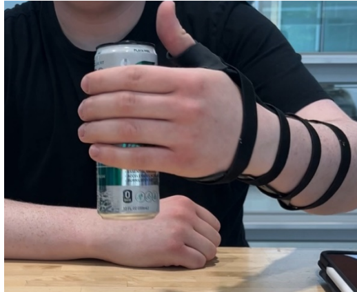
Figure 5: Platform attachment assisting in holding a can without the use of the thumb.
