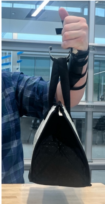
Figure 7: J-hook attachment lifting a lunchbox.
